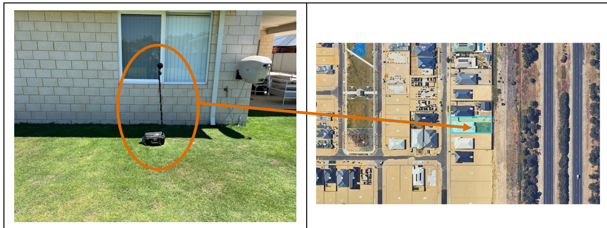
Figure 3-1: Location of Noise Logger on Site
