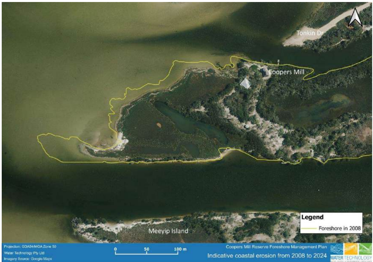
Figure 2-16 Indicative coastal erosion between 2008 and 2024. The yellow outline shows where the foreshore was in 2008 in comparison with the satellite image taken in November 2024 (Metromap). This is indicative and water level comparisons and adjustments have not been made.
