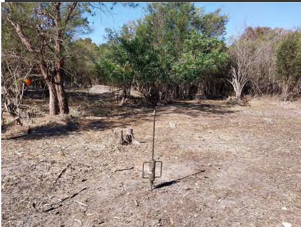
Photo 6. Test Location 04 (PSP4), Testing by Using a Perth Sand Penetrometer
