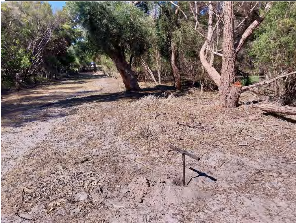
Photo 5. Test Location 04 (TH4), Sub-surface Probing by Using a Hand Auger
