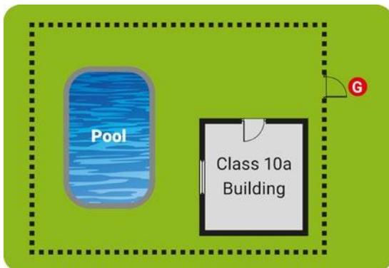
The Class 10 building is wholly within the pool area and does not provide access to the pool through the safety barrier. As the building is not habitable, access between it and the pool does not need to be restricted.
