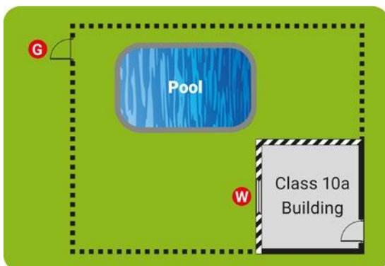
The Class 10 building forms part of the safety barrier. The openable portion of the window must be child-resistant, otherwise the Class 10 building provides access into the pool area through that window. The door does not form part of, and is not generally permitted to be part of, the safety barrier and as such does not need to be restricted.
