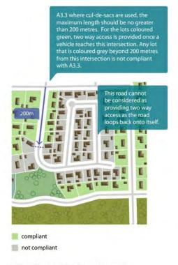
Figure 21: Example of compliant and non-compliant two-way
