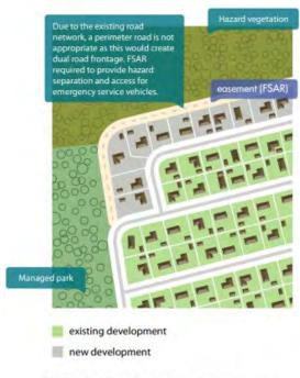
Figure 26: Example of a fire service access route
