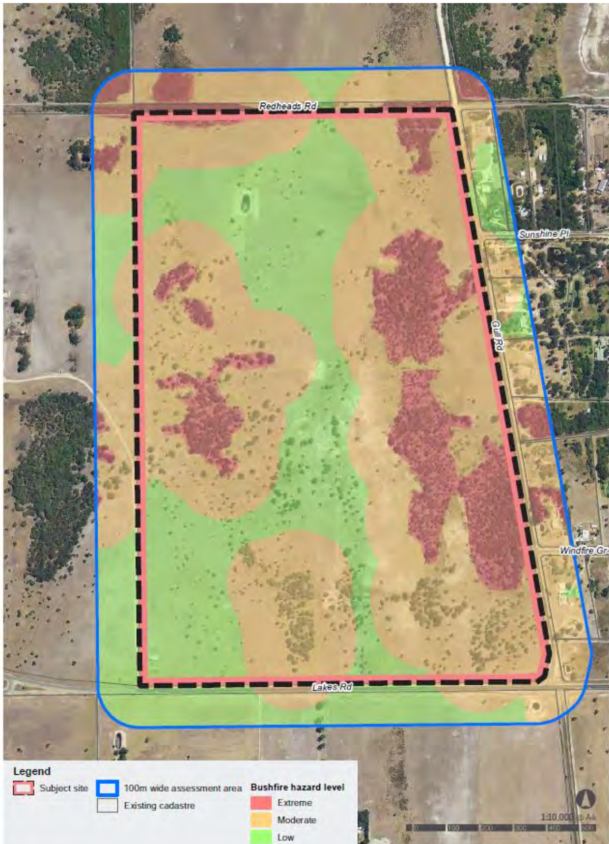
Figure 10 – Bushfire Hazard Level Assessment
