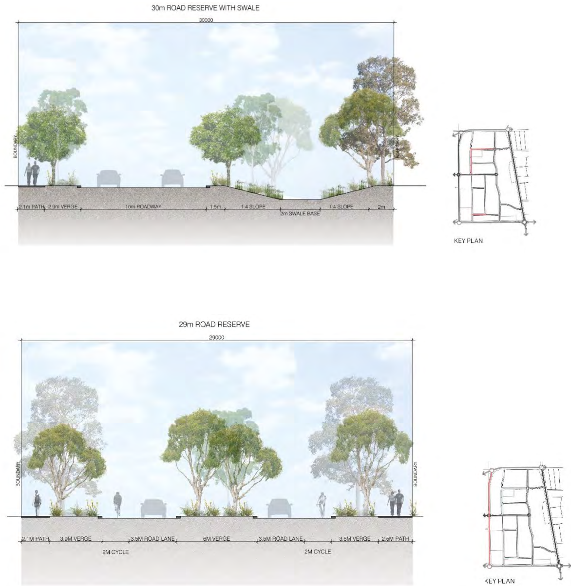
Figure 20(a-f) – Road Cross-sections
