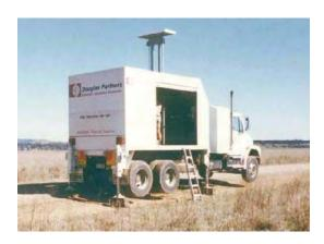
Figure 2: Purpose built CPT rig
