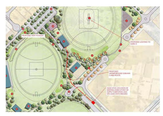
A single new external switchboard is proposed to be utilised to supply both the new clubrooms, and the new oval lighting.
