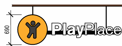
S2 PLAYPLACE 1: 50 YELLOW LOGO WITH INDIVIDUAL POLYCARBONATE LETTERING FIXED TO FRAME. INTERNALLY ILLUMINATED. WHITE LETTERS.
