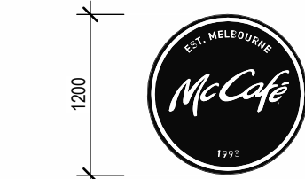
S5 McCAFE WALL BUTTON SIGN 1: 50 FABRICATED METAL BUTTON SIGN. OPAL FACES WITH BLACK VINYL GRAPHICS. LED ILLUMINATION.
