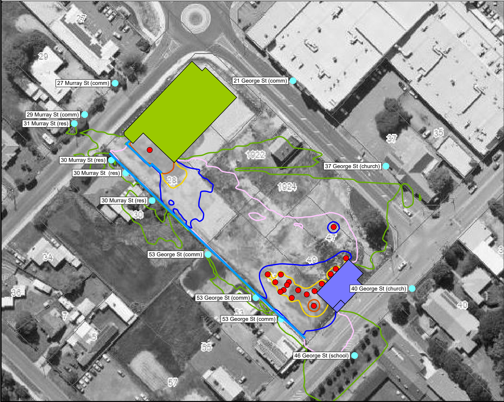
Figure 4-2 Night Noise Contour Plot (1.4m AGL), dB LA1
