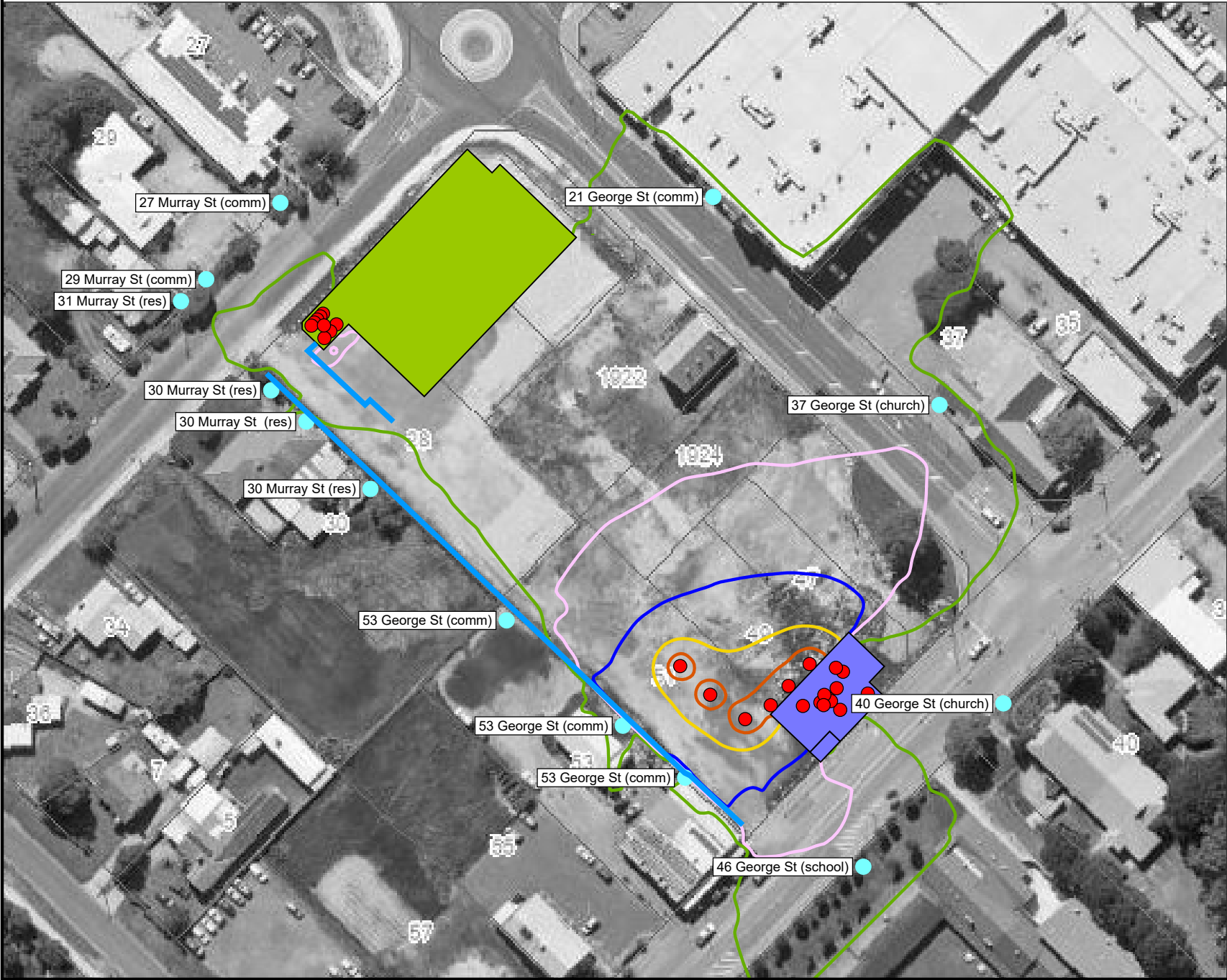
Figure 4-1 Night Noise Contour Plot (1.4m AGL), dB LA10
