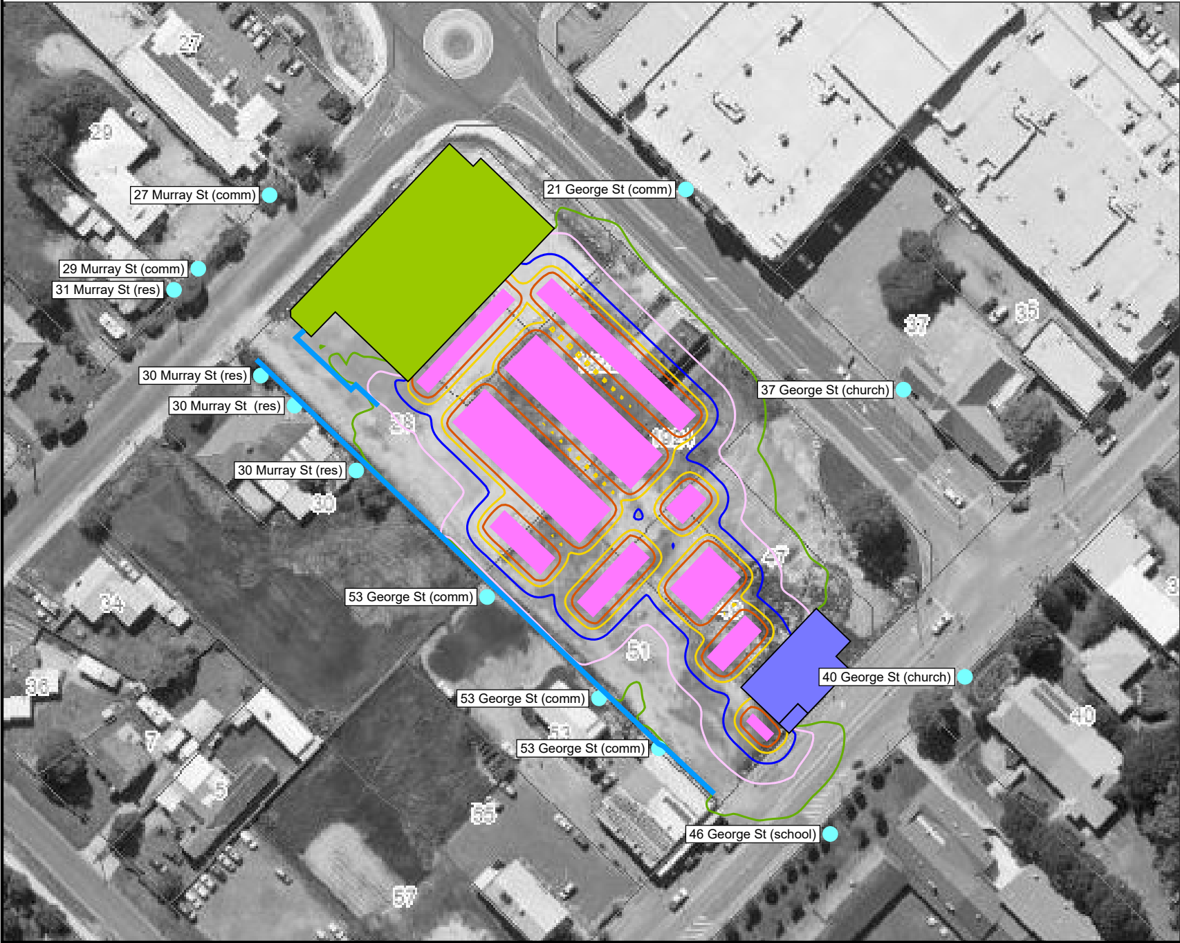
Figure 4-4 Night Noise Contour Plot (1.4m AGL), dB L Amax
