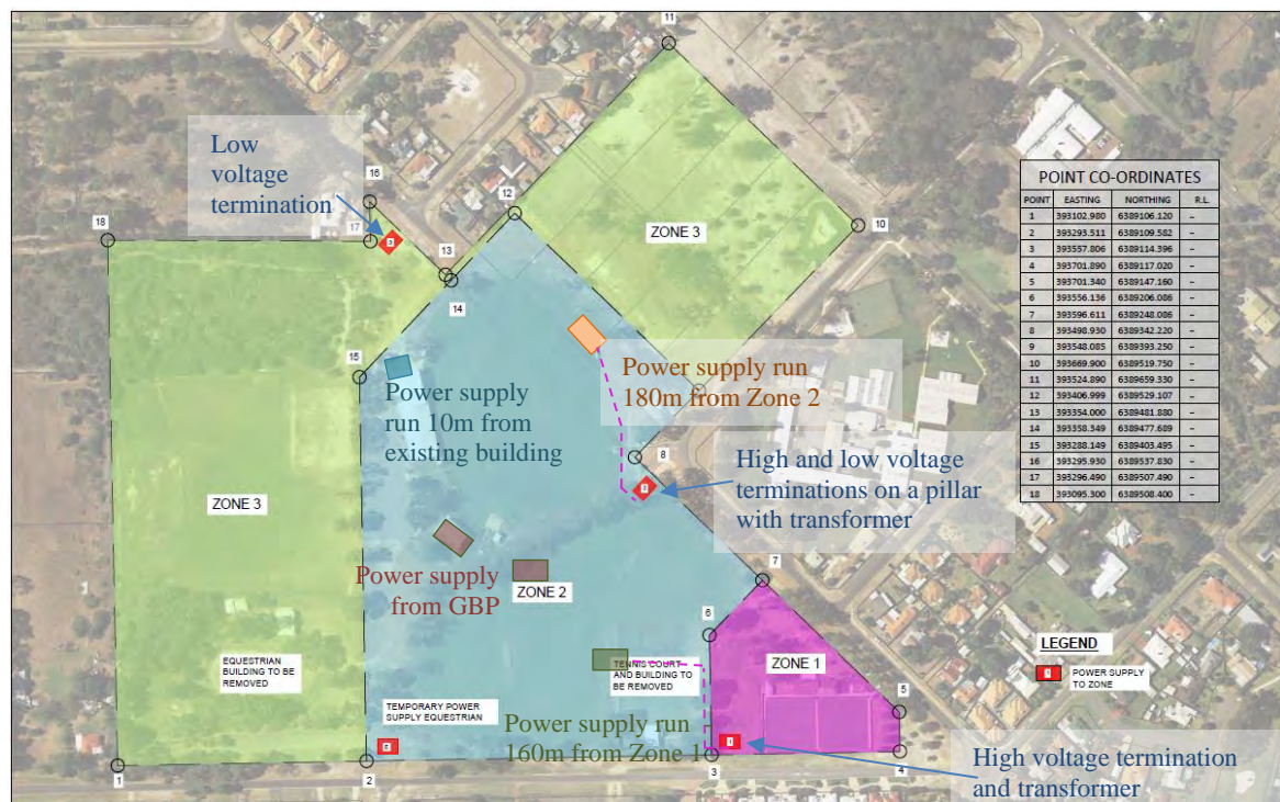
Figure 9: Electrical supply zones at SRMSP
