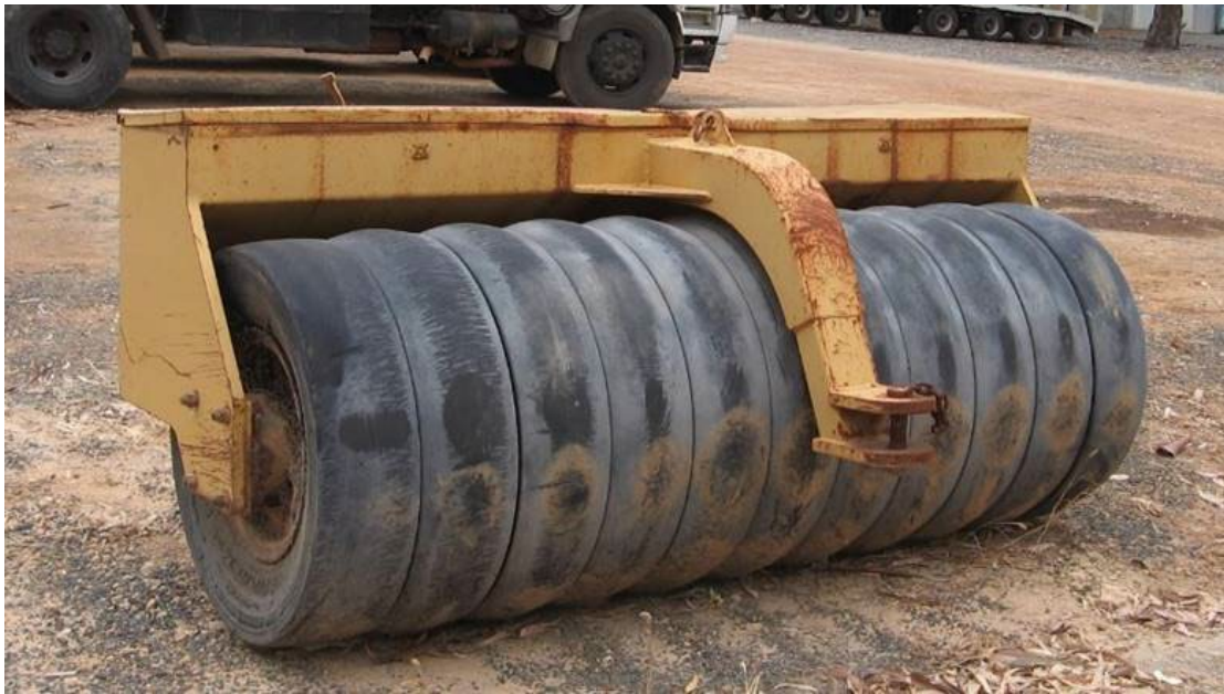
Existing maintenance grader roller
